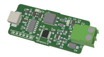
TDFA60250 is a USB voltage meter designed for reading analog voltage signals in the range of 0-5V or 1-5V. It can acquire voltage data in real-time at a speed of up to 1,000 samples per second with a resolution of 12 bits (4,096 levels). It's important to note that the circuits on the USB side and the measurement side are electrically isolated for safety. Additionally, it operates on bus power, eliminating the need for an external power source.
